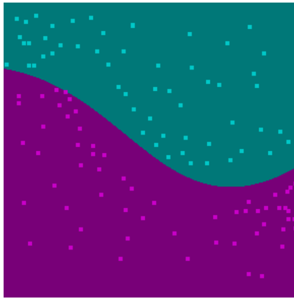
Fig. 7. An illustration of how Support Vector Machines divides data into two separate regions. This example is one for which the data is perfectly separable.
